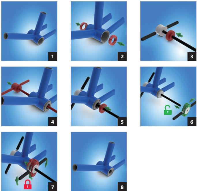
We determine the correct adapter (C) size by inspecting the bearing we will install. We either search by the bearing standard such as 6802 for example, or we take a vernier and measure inner and outer dimension of the bearing. Adapter 25 x 14, where 25 represents the outer dimension of the bearing and 14 represents the inner dimensions of the bearing, in mm.
